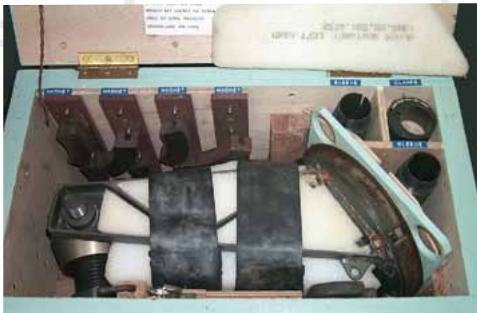
BOX 1, NSN 1385-99-533-1203 contains the stand, buoyancy blocks, spare accessories and maintenance tools.
