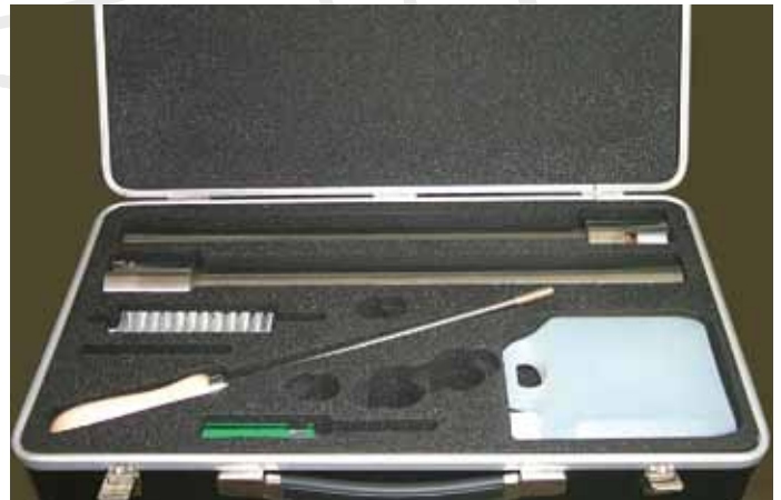
BOX 2, NSN 1385-99-965-7250 contains 2 barrel and breach assemblies, cleaning brush, water container, screwdriver and operators handbook.
